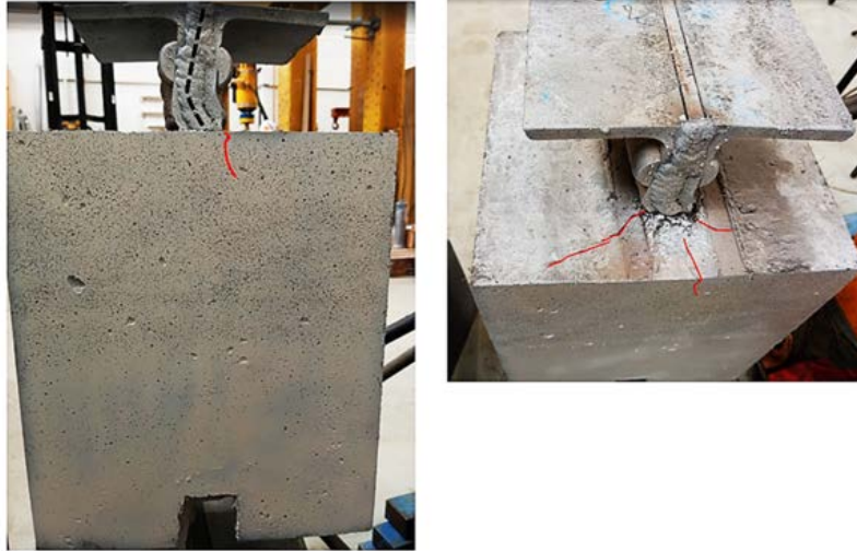
Fig. 17: Local web buckling and surface cracks initiating near the rivets and at the web–UHPC geometric discontinuity, propagating toward the outer surface of the UHPC.
